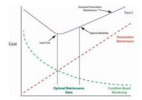
Figure 2. Condition monitoring using balanced approach
